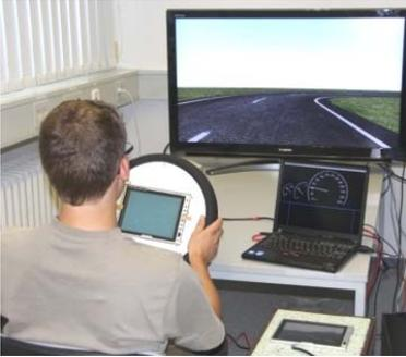
Figure 1. Study setup. Touchscreen displays on the steering wheel and in the middle console serve as input and output interfaces. Laptop serves as dashboard display (and speedometer). Large display shows first person view of the driving simulator.
