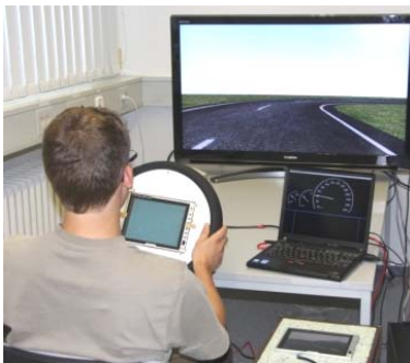
Figure 1. Study setup. Touchscreen displays on the steering wheel and in the middle console serve as input and output interfaces. Laptop serves as dashboard display (and speedometer). Large display shows first person view of the driving simulator.
