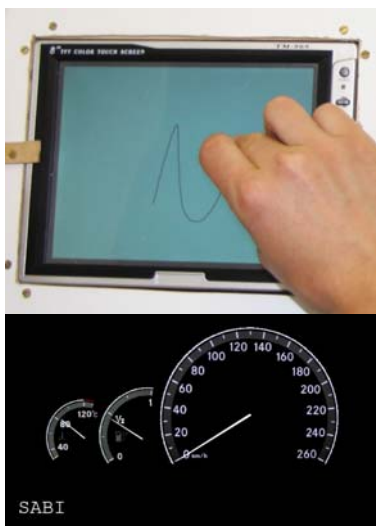
Figure 3. Graphical User Interface of the prototype indirect feedback . Recognized characters shown on the dashboard screen.
