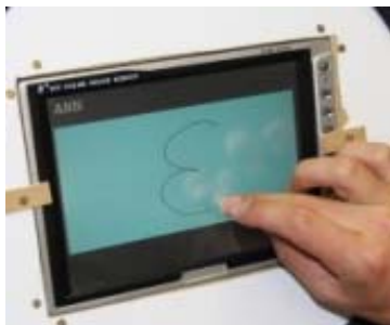
Figure 2. Graphical User Interface of the prototype direct feedback . Recognized characters are shown above the input area.
